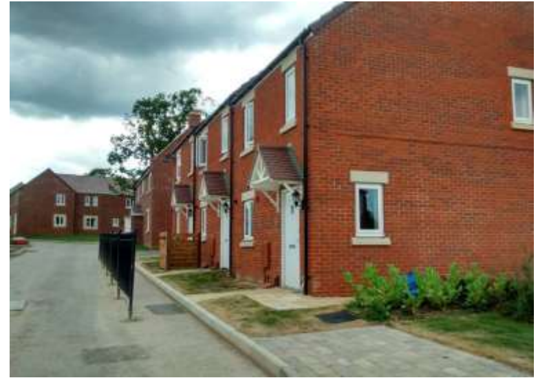
Figure 23-24. Strange edge condition between pavement front entrances and road. An unusual fence has been erected to enable safe pedestrian access but illustrates poor planning.
