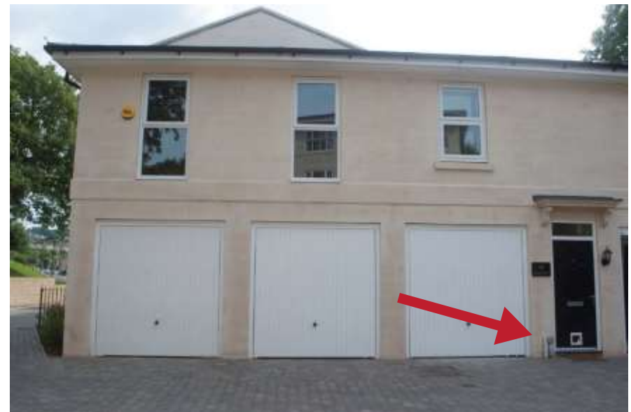
Figure 7. Front door is directly next to garages with no distinction in zones. Lack of soft landscaping or distinction in materiality creates an abrupt transition between public and private areas.
