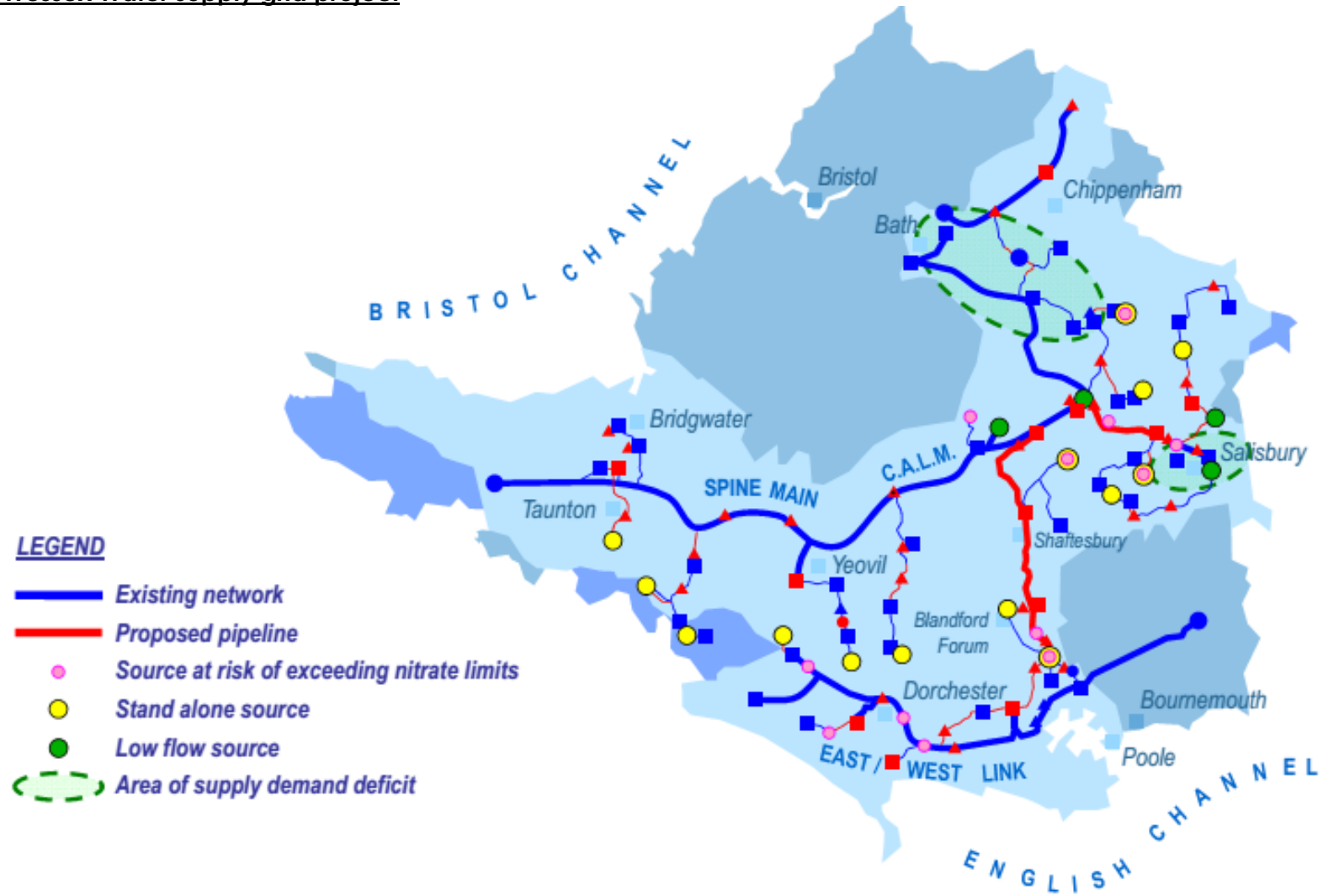
Figure 19: Wessex Water supply grid project
