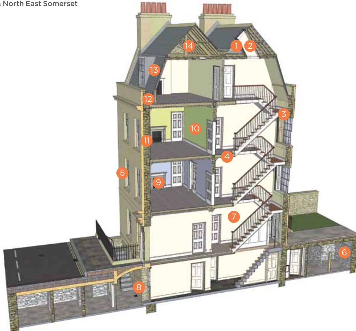
Section drawing of a typical 18th Century Georgian house in Bath & North East Somerset
