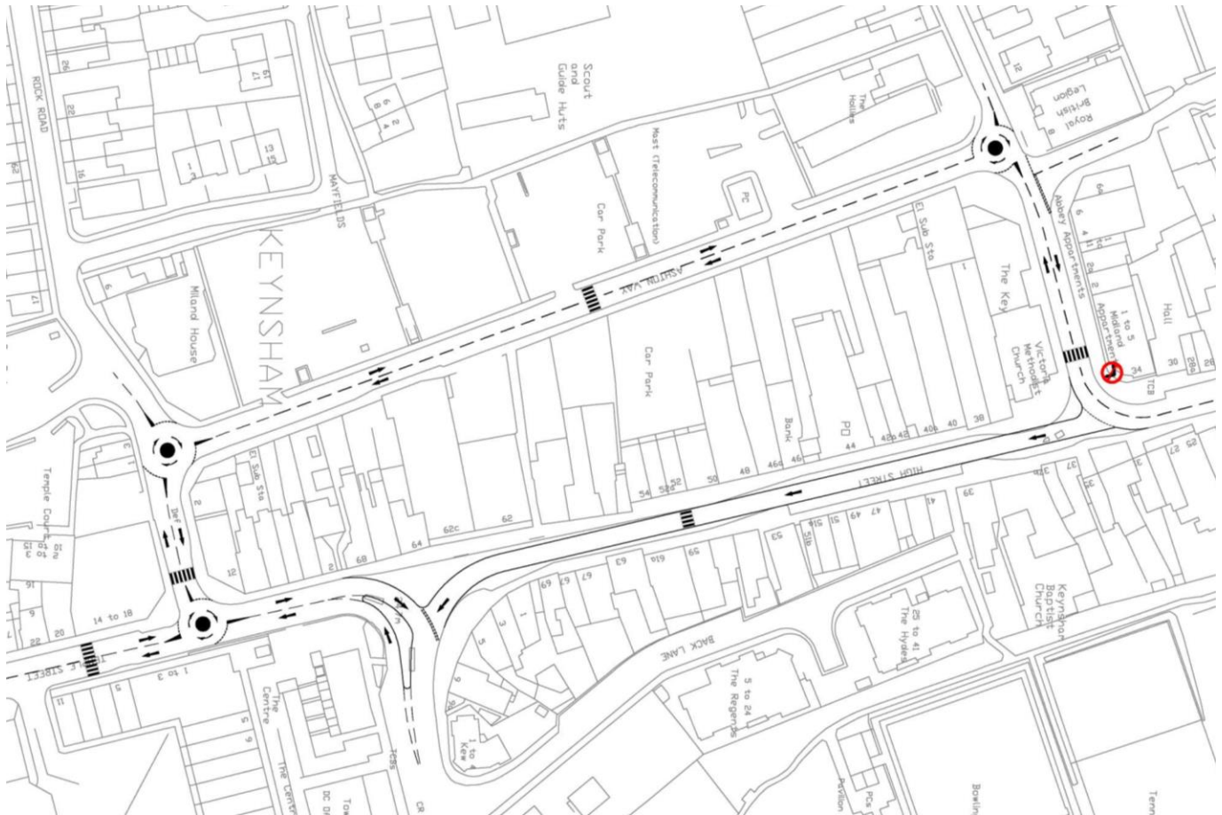
Figure 2.18: One-way High Street southbound
