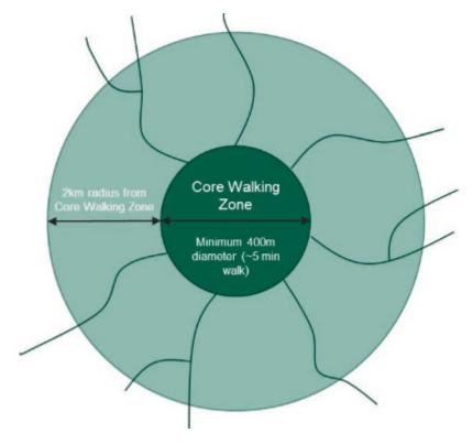
A Core Walking Zone is an area with a minimum diameter of 400 meters, which equates to an average walking time of about 5 minutes. Within these core zones all pedestrian infrastructure is considered crucial to providing safe journeys for people walking and wheeling. An outer 2km radius from the core walking and wheeling zone boundary has then identified. This area encompasses the important pedestrian routes that serve the core walking and wheeling zone.
