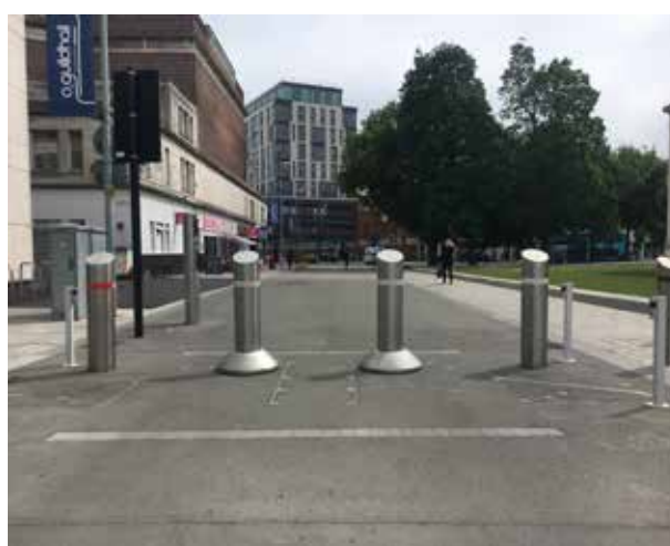
Moving bollards in Southampton
