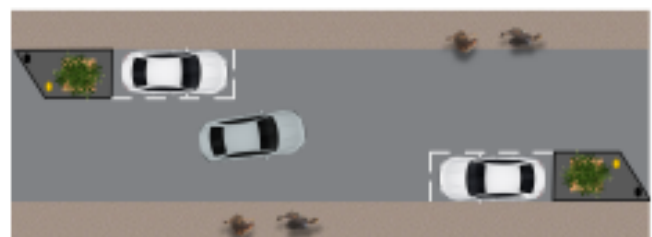
Chicane parking arrangement with build outs
