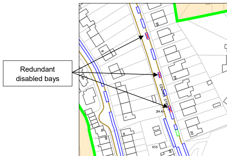
Figure 5: Edward Street redundant disabled parking bays
