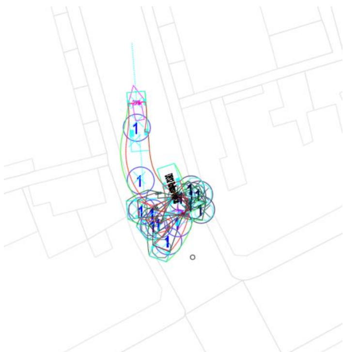
Figure 13: Refuse Vehicle Tracking Movement encroaching on footways
