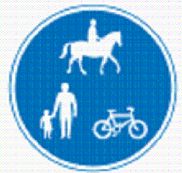
Figure 11-19 Diagram 956.1 (S3-2-30) Route for use by pedal cycles, horses and pedestrians only
